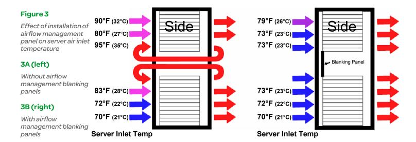
The summary of this data is presented in **Table 3**. The data shows that the coolest servers are located at the bottom of the rack and are unaffected by the use of the airflow management panel. The hottest server is located just above the unused and open vertical rack space and experiences an inlet temperature reduction of over 20°F (over 11°C) when the airflow management panel is installed.
